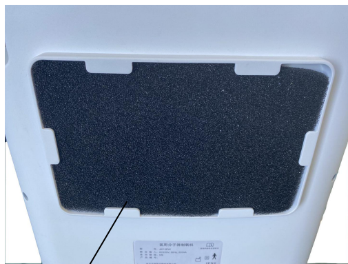
Intake air filter
